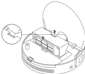
2. Open the dust compartment cover, and empty out the contents.
