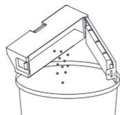
Note: To prevent the filter from becoming clogged, lightly tap the dust compartment when emptying its contents.
