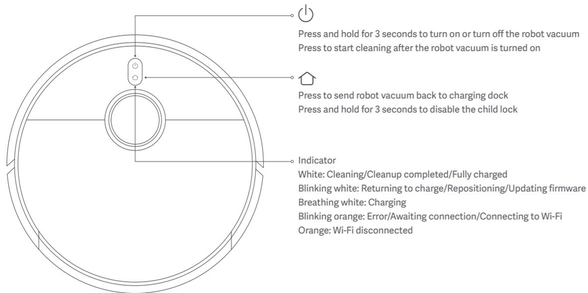
Note: When the robot vacuum is cleaning or returning to the dock to charge, press any button to pause it.
